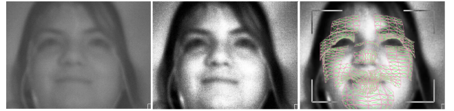
Fig. 6. Participant’s facial video before (left) and after (middle) histogram equalization. Tracking 3D grid is shown on the right.
